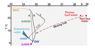
Fig. 12.5. T-S diagram showing the source water masses for the Indian Ocean and their effect on the temperature - salinity structure in different regions. Curve *a* is representative for the region between Australia and Indonesia (120°E), curve *b* for the Bay of Bengal (88°E) to 10°S, curve *c* for the subtropics south of 10°S. Intrusions of Red Sea and Persian Gulf Water can produce departures from the T-S curves near the isopycnal surface  $\sigma_t = 27.2$  (the "mixing line").
