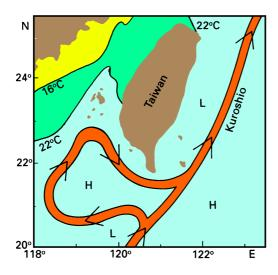
Fig. 10.15. Sea surface temperature and inferred flow direction in Taiwan Strait on 8 January 1986. Observed differences in steric height between high (H) and low (L) sea level are of the order of 0.15 m. Adapted from Wang and Chern (1988).
