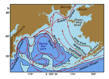
Fig. 10.1. Surface currents in the Bering Sea. Shading indicates water depth less than 3000 m; in the region of the Bering Slope Current the 200 m isobath runs close to the 3000 m isobath. The Shirshov Ridge is seen near 171°E, the Bowers Ridge north of the Aleutian Islands near 180°.
