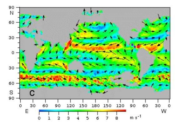
Fig. 1.2. Surface winds over the World Ocean. (a, page 4) Annual mean, (b, page 4) July mean, (c) January mean. Data from <u>http://ferret.wrc.noaa.gov/las/</u>, the NOAA Live Climate Data Server using the Comprehensive Atmosphere/Ocean Data Set (COADS) climatology. COADS is based on ship observations; regions without data are gray. Colour indicates wind speed.
